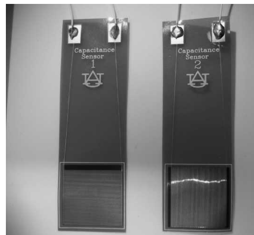
Fig. 3. Photograph of the horizontally arrayed sensor (left) and the vertically arrayed sensor (right).
