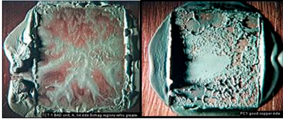
Fig. 3. Images of thermal greases after temperature cycling and disassembly of the package. The image on the left shows evidence of pump-out, whereas the image on the right shows no evidence of pump-out (adapted from [31]).
