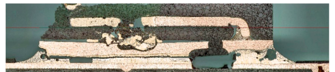
Fig. 3. Cross-sectional image of an electrically failed device after the EM test.
