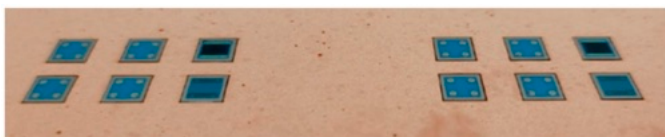
Fig. 17. Ceramic platelets ( 5 \times 5 \times .6 \text{ mm}^3 ) integrated in and electrical contacted with the PCB substrate ( 303 \times 227 \text{ mm}^2 ) using the sinter lamination technology.
