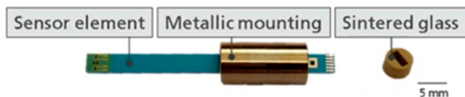
Fig. 21. Ceramic sensor element with metallic mounting.
