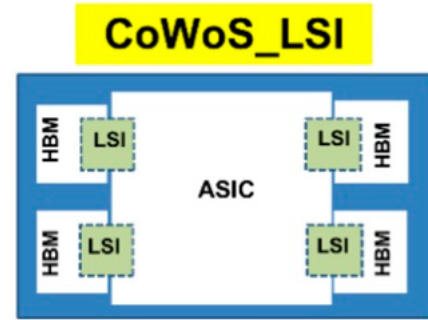
Fig. 33. (a) TSMC's InFO-LSI. (b) CoWoS-LSI.
