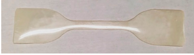
Fig. 4. Test specimen according to DIN EN ISO 527-3 [8] with the shape of type 5 and thickness of 200 \mu\text{m} .
