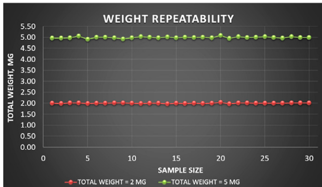
Fig. 8. Weight Repeatability for a piezo-driven valve.
