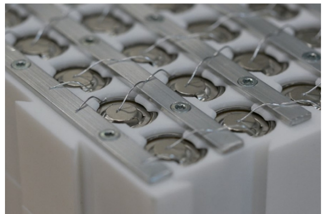
Figure 1. Aluminum wire bonded battery module.
