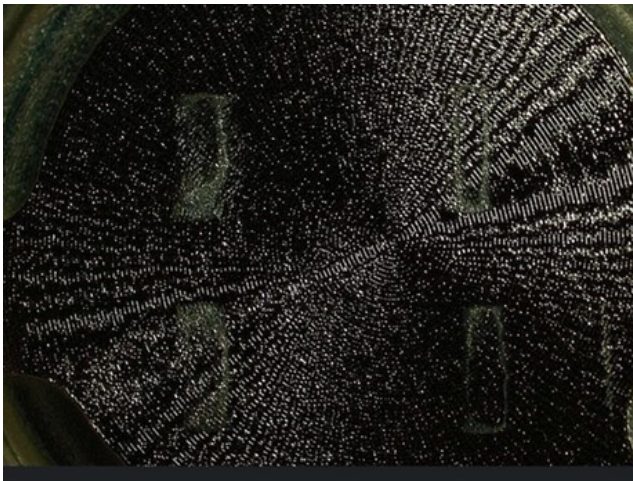
Figure 8. Unacceptable shear nuggets of four welds.
