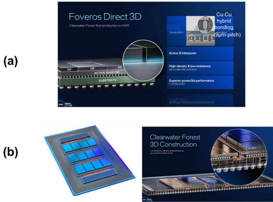
Figure 15. Intel's Clearwater Forest with Hybrid Bonding
