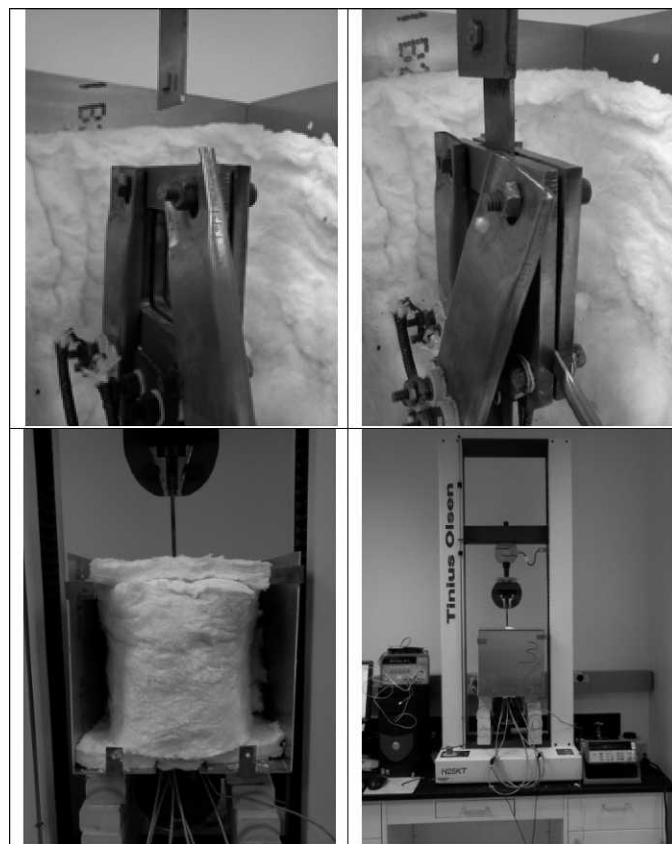
Fig. 14. High temperature shear test system: integration of a miniature oven in a benchtop testing machine.
