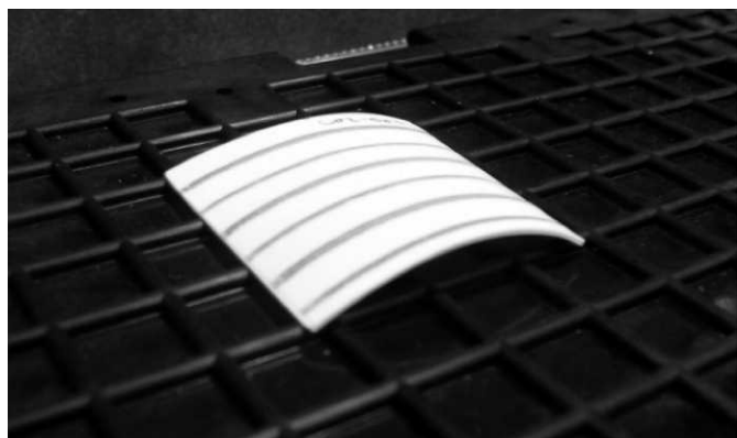
Fig. 8. Bending effect of C02 silver lines on a cofired ceramic (2 in × 2 in).
