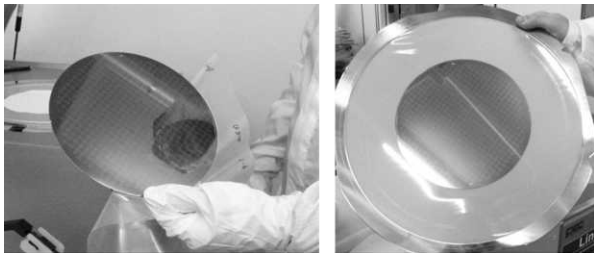
Fig. 17. Removal of protective film from wafer with WAUF and placement of dicing tape.
