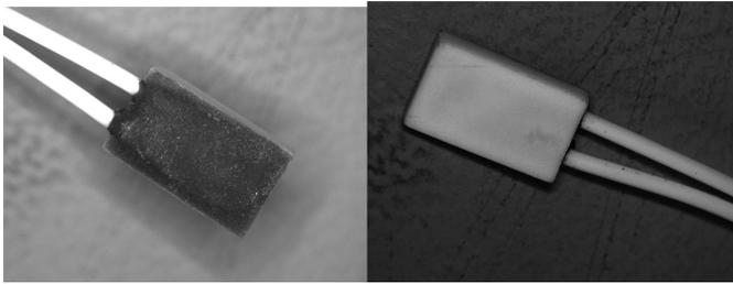
Fig. 19. Photographs of the temperature sensor/PRTs (Type Y) to be used for the MSL project.
