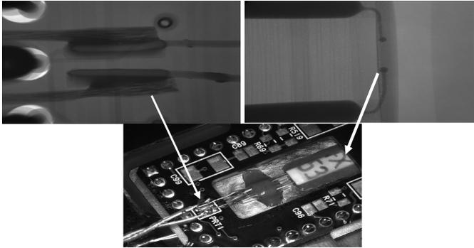
Fig. 20. X-ray images and an optical image of the PRTs that used in MSL engineering camera.
