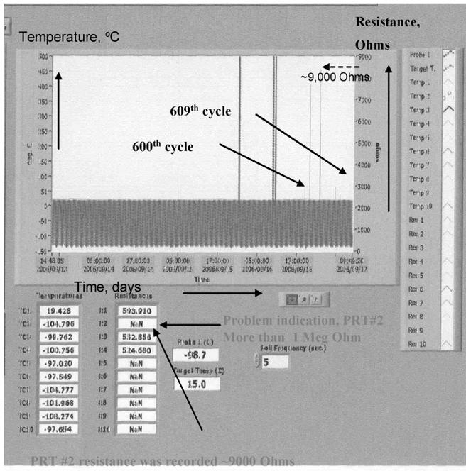
Fig. 21. Showing the signs of PRT (Type X) failure at 585th thermal cycle and continued until 609th thermal cycle.
