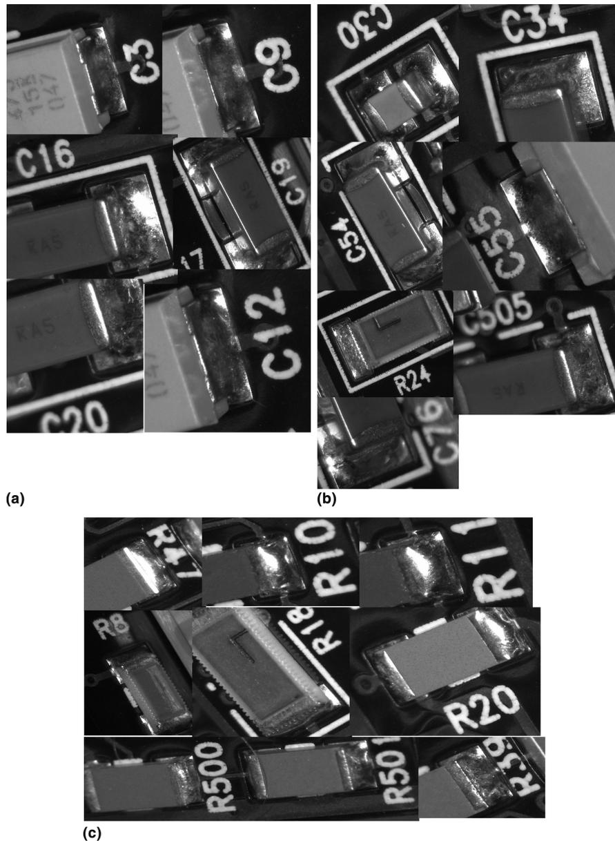
Fig. 18. Photographs of the capacitor solder joints and resistor solder joints taken after 2010 thermal cycles.
