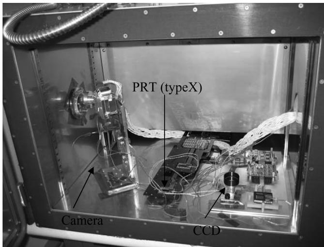
Fig. 7. Photograph of the MSL engineering camera in the side thermal chamber, electronics board, PRTs, CCDs, and so on.
