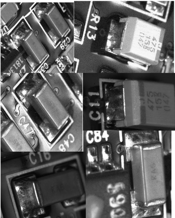
Fig. 15. Photographs of the capacitor solder joints and resistor solder joints taken after 1005 thermal cycles.
