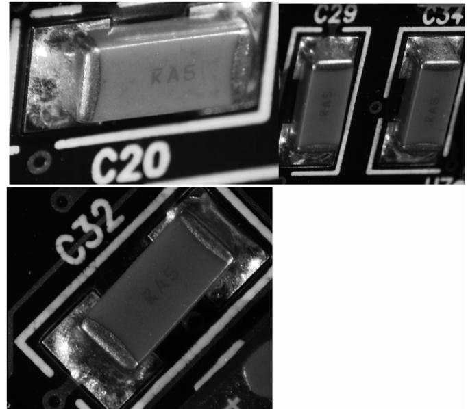
Fig. 13. Photographs of the capacitor solder joints after just 15 thermal cycles.
