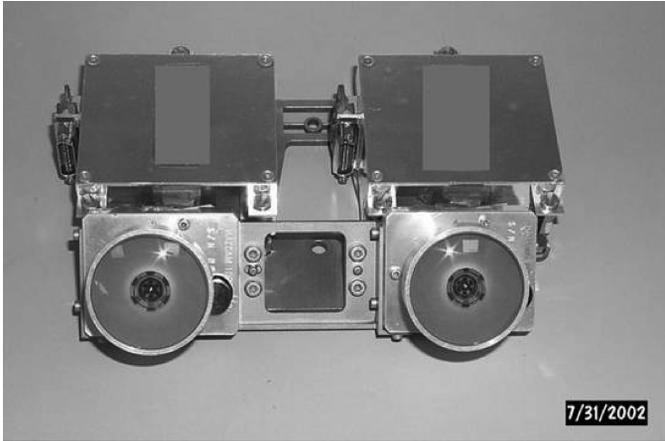
Fig. 1. Optical photograph of the engineering camera that was used in MER project.
