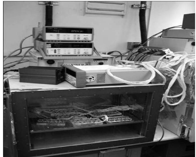
Fig. 23. PRTs (Type Y) under the extreme temperature thermal cycling test.
