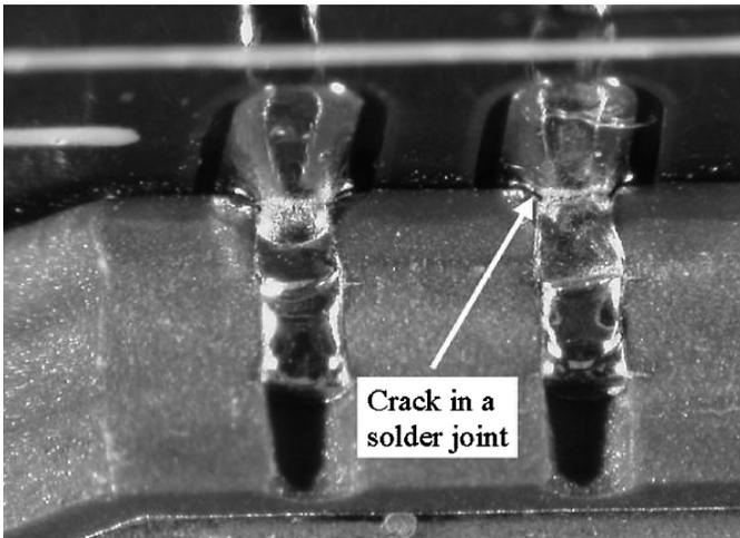
Fig. 3. Optical photograph of a cracked interconnect in a package assembly after 50 cycles with a  $\Delta T$  of 235°C (–120°C to 115°C) for the MER mission.
