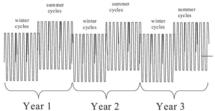
Fig. 6. Sequence of thermal testing profile for the MSL mission.
