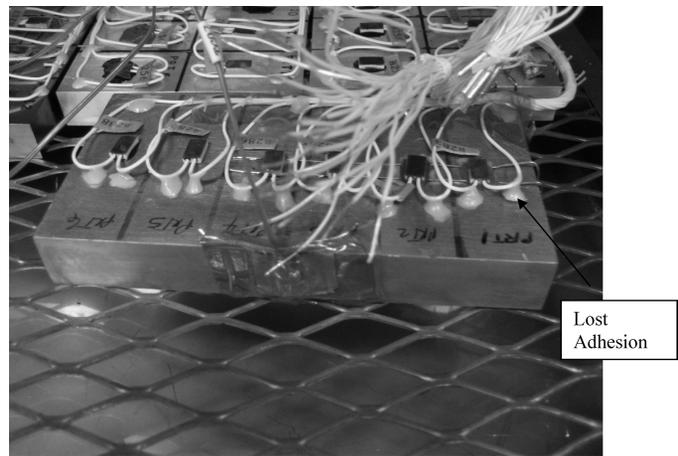
Fig. 25. Loss of adhesion of stacking materials as a function of thermal cycling.
