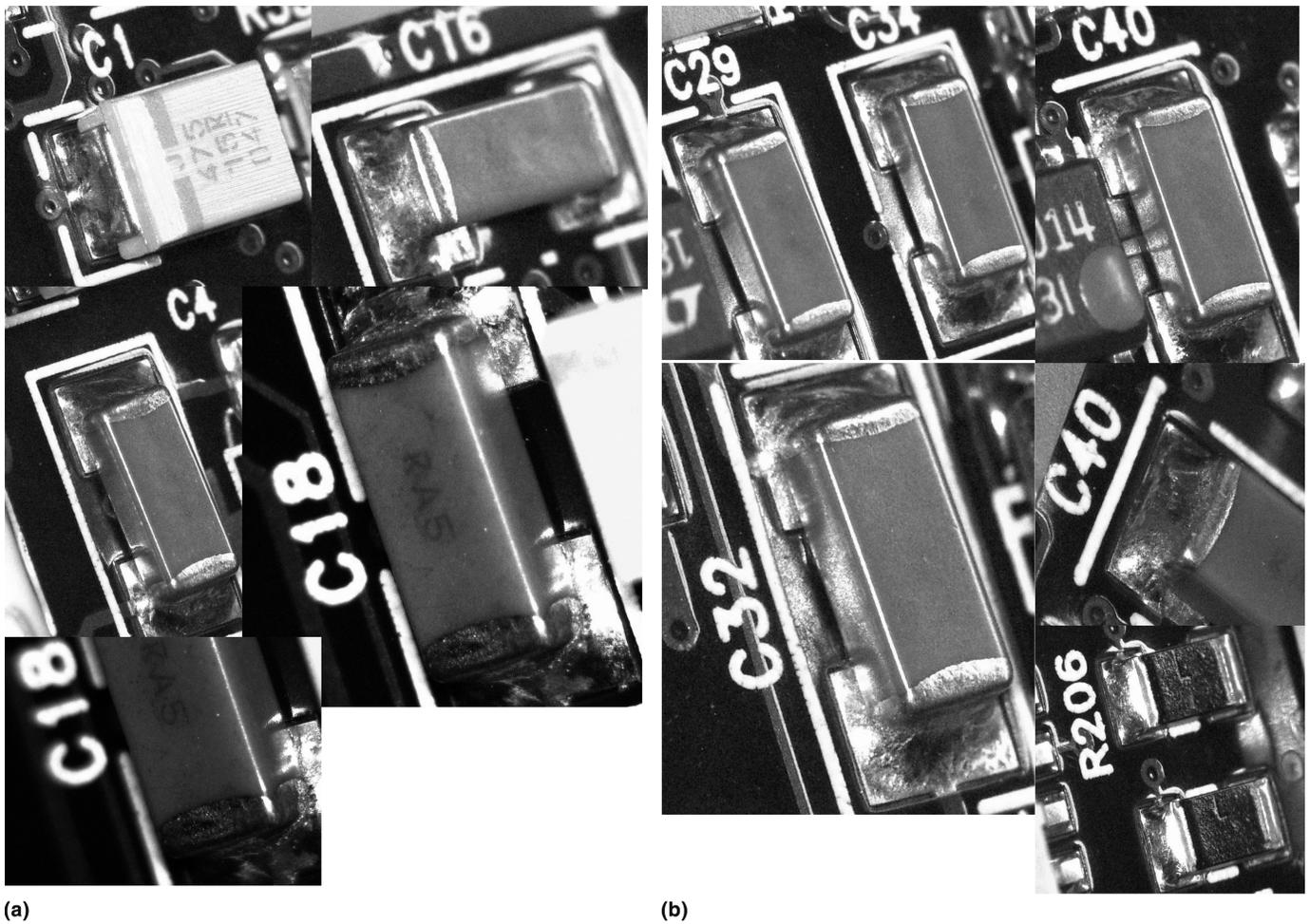
Fig. 17. Photographs of the capacitor solder joints and resistor solder joints taken after 1675 thermal cycles.
