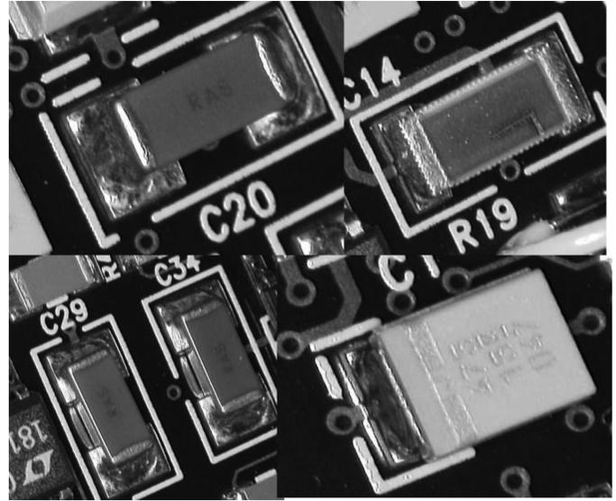
Fig. 12. Photographs of the capacitor and resistance solder joints prior to thermal cycling.
