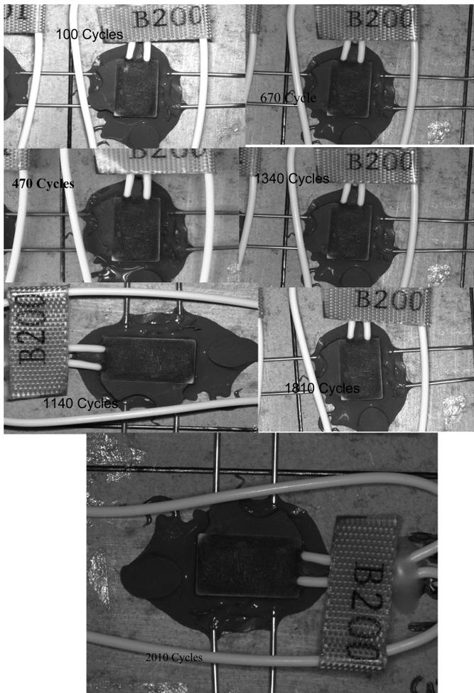
Fig. 24. Photographs of the PRTs that were taken as a function of number of the MSL thermal cycles.
