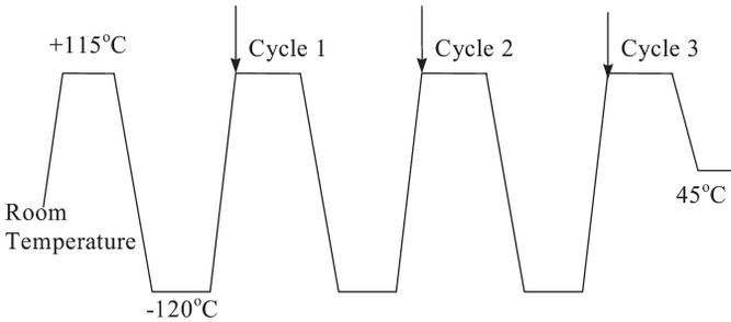
Fig. 2. Temperature profile used for MER mission to qualify the packages.
