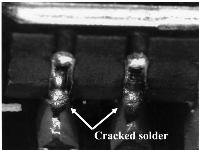
Fig. 8. Photograph of a cracked interconnect in a leadless package of camera assembly after 170 cycles with a  $\Delta T$  of  $145^{\circ}\text{C}$  ( $-105^{\circ}\text{C}$  to  $40^{\circ}\text{C}$ ) for the MSL mission.
