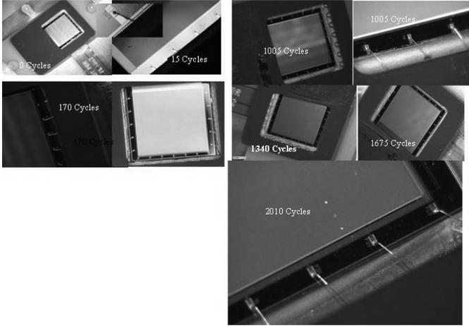
Fig. 11. Photographs of the wire bonds in the CCD as a function of various thermal cycling stages.
