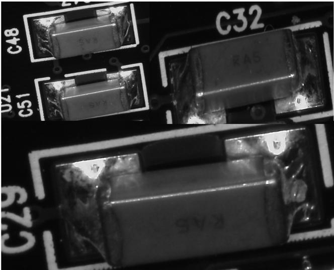
Fig. 14. Photographs of the capacitor solder joints taken after 170 thermal cycles.
