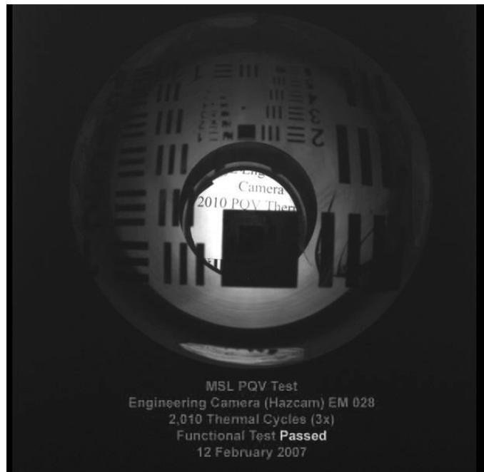
Fig. 9. Images of the test object after complete PQV test.
