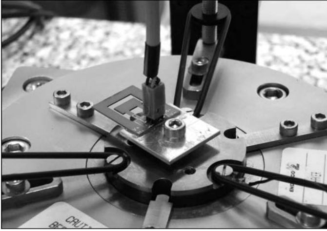
Fig. 11. The accelerometers were characterized by a Spektra vibration exciter.
