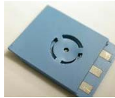
Figure 10. Sintered sensor displaying sagging.
