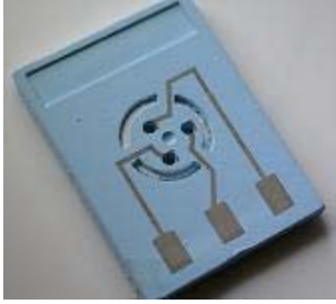
Figure 12. External electrode sensor in green (unfired) state.
