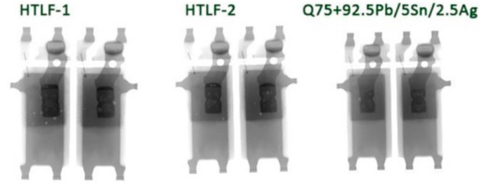
Fig. 3. Voiding performance of both HTLF pastes (HTLF-1 and HTLF-2) and Pb92.5/Sn5/Ag2.5 under the same high-Pb reflow profile with a peak temperature of 385°C.
